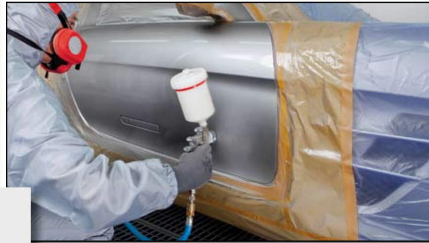
Applying the 2K Special Matt ready to use clearcoat mixture in two carefully controlled overlapping coats with inter-coat flash-off.
