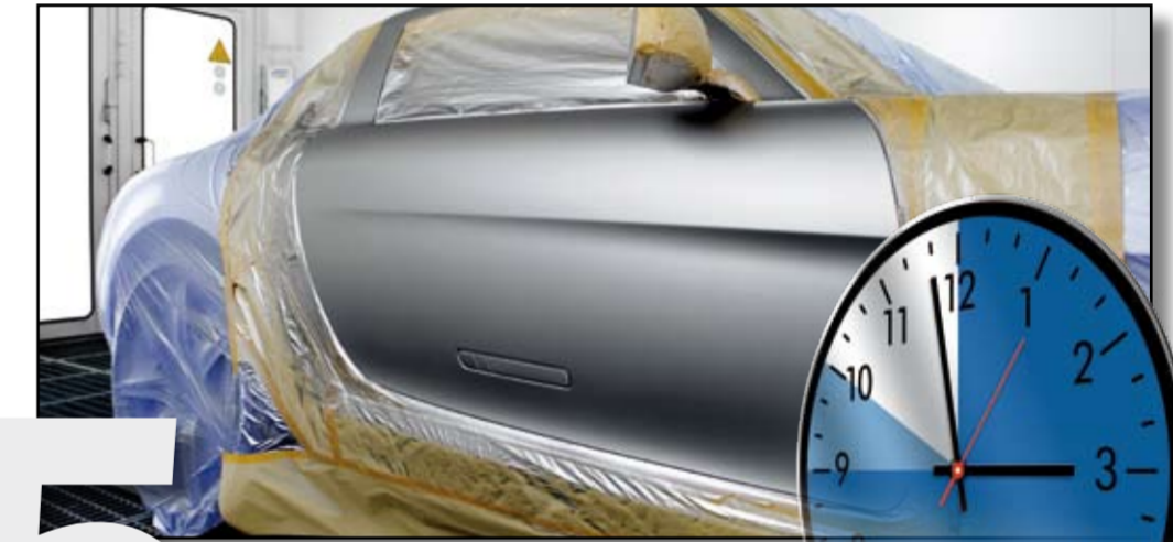
Drying the matt clearcoat 45 - 50 minutes at 60 °C.
